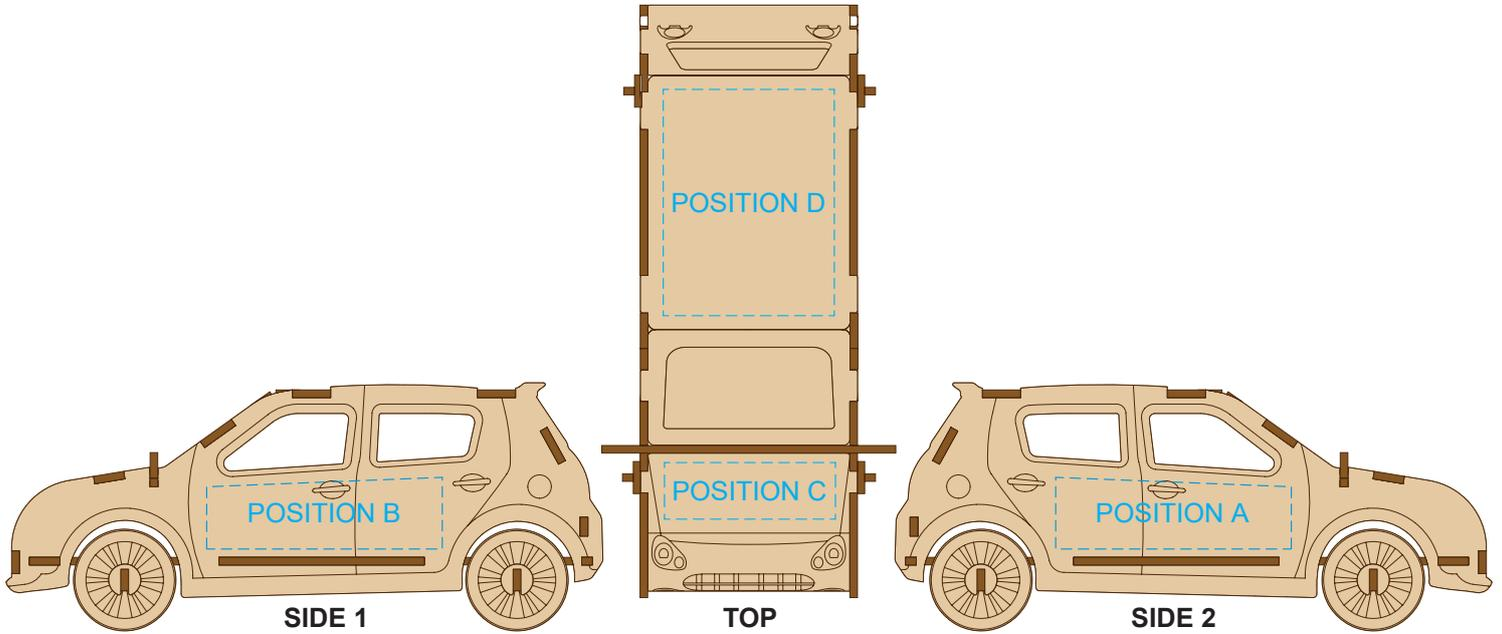
Up to a 2mm tolerance is expected for alignment of the printed artwork against the engraved lines. Slight inconsistencies are to be considered acceptable if the artwork is printed over an engraved line.
